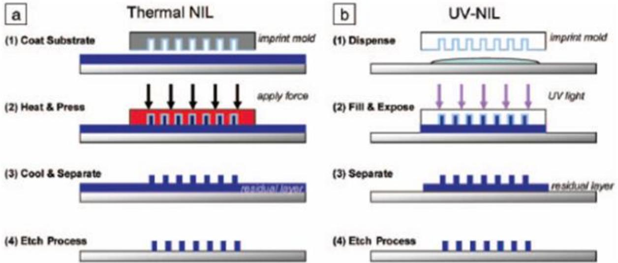
Figure 2 Two fundamental process types of NIL (Steward & Wilson, 2005)
