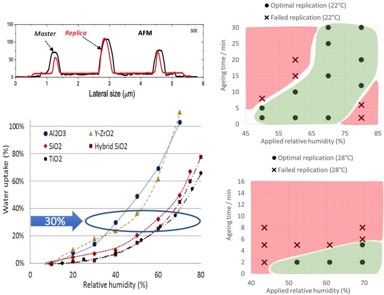
Figure 6: (bottom-left) In situ ellipsometry investigation of plain Sol-gel films swelling vs. applied humidity. (Right) processability of  $\text{TiO}_2$  sol-gel with respect to humidity, temperature and waiting time after liquid deposition. (top left) AFM profiles of features present on the silicon master and obtained after replication in silica.
