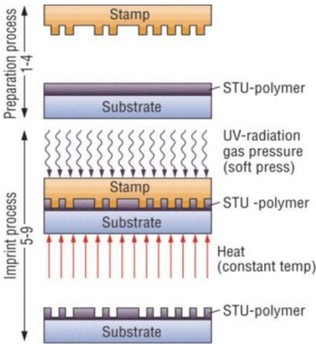
Figure 3. A simultaneous thermal and UV (STU) imprint process
