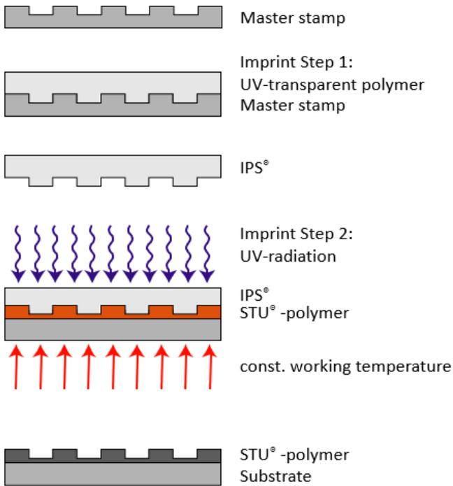
Figure 4. Imprint process with an Intermediate polymer stamp
