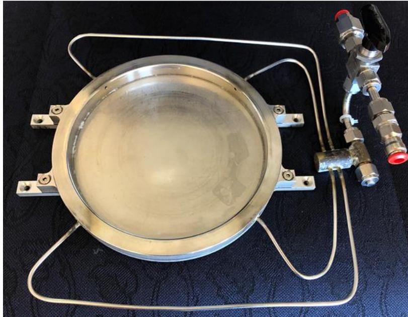
*Figure 7: Humidity control chamber used during the nanoimprint process, the high humidity water can be introduced into the chamber by inlet.*
